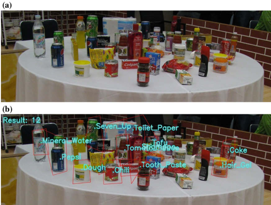
Fig. 12 The input image for object recognition as acquired by our robot during the Technical Challenge of the RoboCup (a) and the output image depicting the recognition results (b). During training and recognition an image resolution of 8 MP was used
