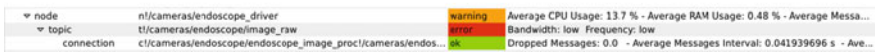
Fig. 14 The orange color of the node shows that a problem had occurred a short while ago, but that the current state is within the specification. When the topic is marked red this means it is currently not working as intended, i.e. violating one of the specifications
