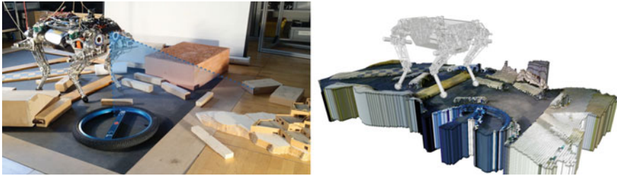
Fig. 10 The quadrupedal robot StarLETH [10] is walking over obstacles by using the elevation mapping node to map the environment around its current position. A Kinect-type range sensor is used in combination with the robot pose estimation to generate a probabilistic reconstruction of the terrain
