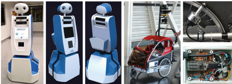
Fig. 2 Left Picture and renderings of the SPENCER robot platform. Right The custom-built mobile data capture platform, including a custom odometry solution using quadrature encoders in dynamo housings on both main wheels, connected to a microcontroller ( bottom right picture ). Both platforms contain numerous ROS-based software components distributed over multiple computers
