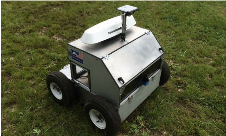
Fig. 5 Scipio autonomous skid steer robot
