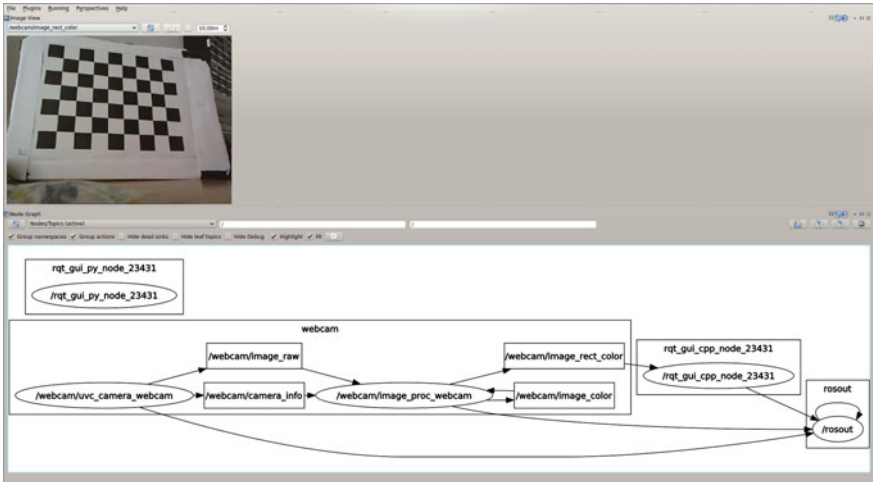
Fig. 2 The screenshot shows rqt with the “Image View” plugin on the top and the “Node Graph” on the bottom . The graph visualizes the simple image processing pipeline consisting of uvc_camera and image_proc
