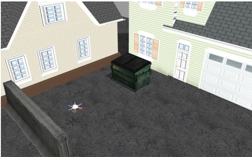
Fig. 1 A screenshot of the RotorS simulator. The scene is built up from Gazebo default models and a Firefly hex-rotor helicopter
