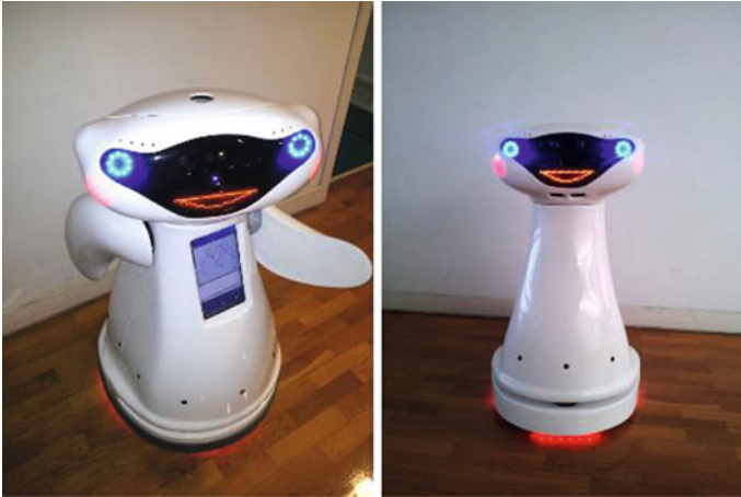
Fig. 2 The two versions of the MONarCH robots: the Socially Oriented (SO) one on the left and the Perception Oriented (PO) one on the right . The core platform is essentially the same, differing only on the set of actuation devices. The SOs are targeted for human-robot interaction, while the POs are targeted to perceive the environment from a mobile platform
