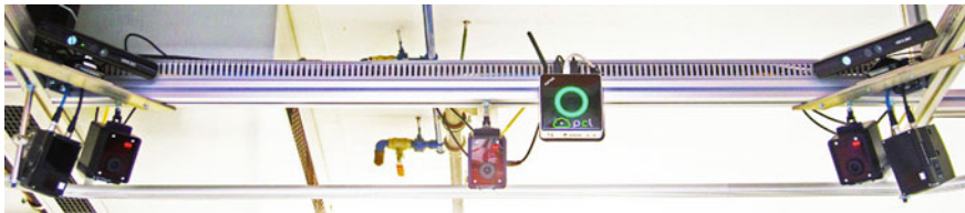
Fig. 4 One side of our sensor rig with different cameras: Kinect (top left and top right), ToF cameras (PMD S3, outermost), optical tracking system (ART, with two visible red LEDs), Kinect server (center, with visible green circle)
