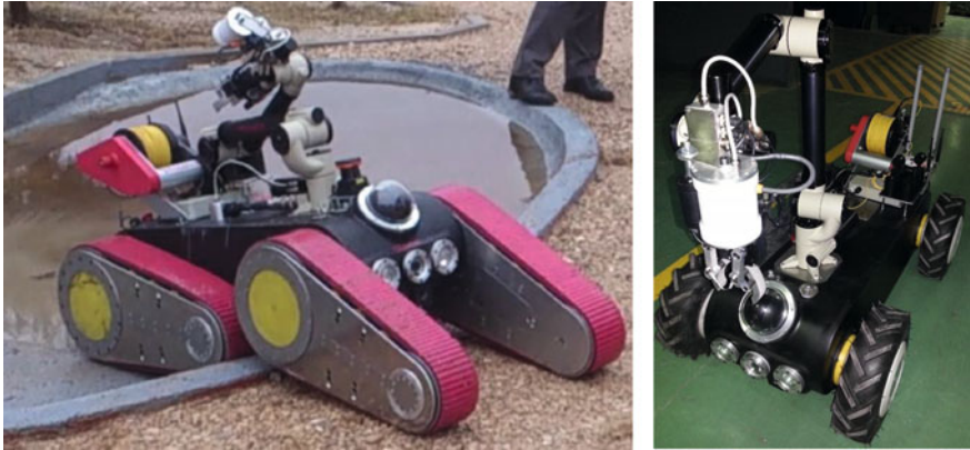
Fig. 1 Rescuer platform with flippers ( left ) and wheel ( right )
