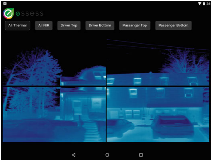
Fig. 8 Operator interface showing thermal camera output
