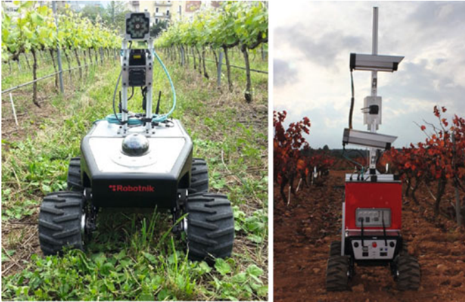
Fig. 24 Vinbot Summit XL HL mobile robot platform testing in vineyards ( left ). Vinbot Summit XL HL platform with mounted precision viticulture sensing unit ( right )
