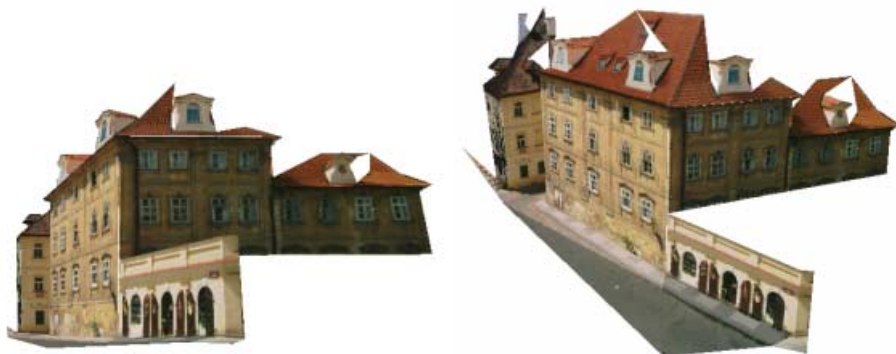
Fig. 5. Two views on the recovered 3D model of the house at Kampa with image texture mapped onto the reconstruction.
