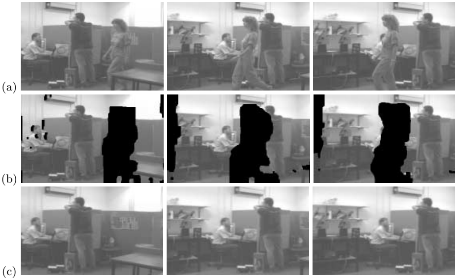
Fig. 3. Dominant motion selection and outlier rejection. (a) 3 representative frames from the sequence. There are two motions present – that induced by the panning camera, and that induced by the walking woman. (b) Outlier pixels detected in those frame are marked in blacks. Those are pixels found to be moving inconsistently with the detected dominant motion. Those pixels correspond to the walking woman, to her reflection in the desk, to the boundaries of the image frames, and to some noisy pixels. (c) Full reconstructions of the dominant layer (the background) in all frames. The girl, her reflection, and the noise are removed from the video sequence by filling in the black regions with gray-level information from other frames according to the computed dominant background motion.
