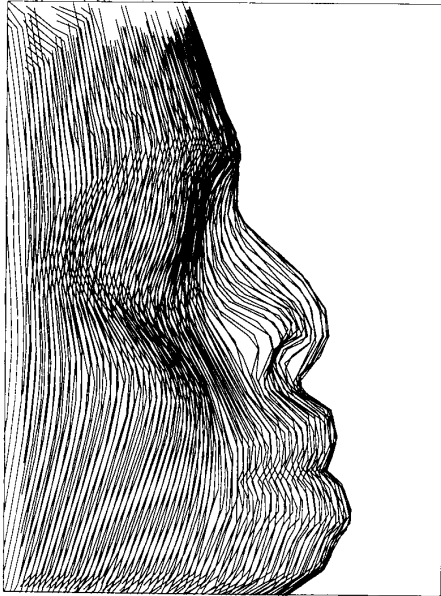
Fig. 14. Side view of range image model and registered point set.
