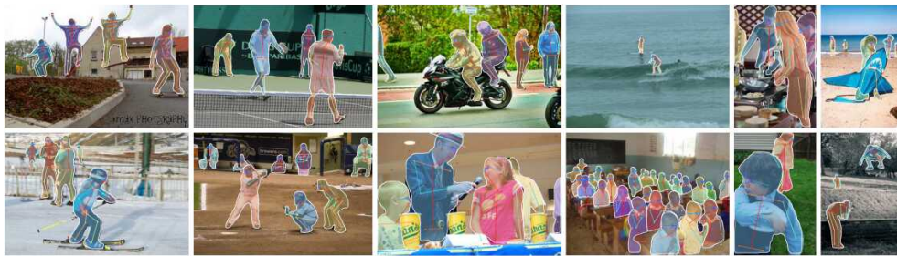
Figure 6.37 Person keypoint detection and segmentation using Mask R-CNN (He, Gkioxari et al. 2017) © 2017 IEEE
