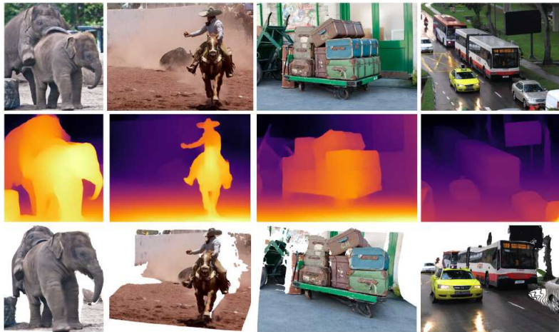
Figure 12.32 Monocular depth map estimates and novel views from images in COCO dataset (Ranftl, Lasinger et al. 2020) © 2020 IEEE.
