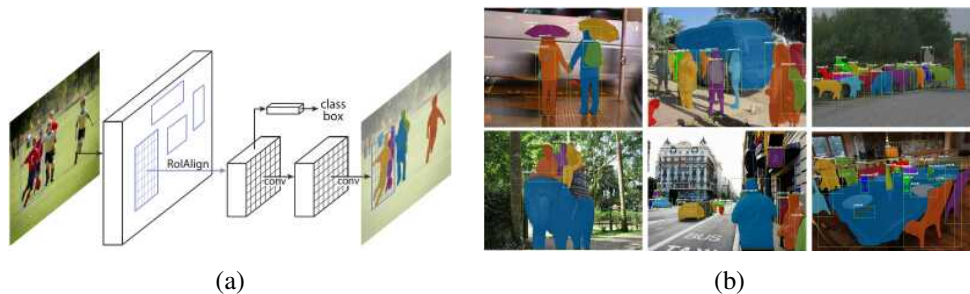
Figure 6.36 Instance segmentation using Mask R-CNN (He, Gkioxari et al. 2017) © 2017 IEEE: (a) system architecture, with an additional segmentation branch; (b) sample results.
