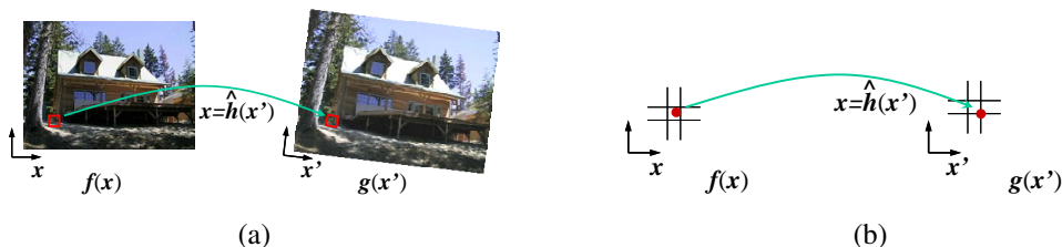
Figure 3.46 Inverse warping algorithm: (a) a pixel g(x') is sampled from its corresponding location x = \hat{h}(x') in image f(x) ; (b) detail of the source and destination pixel locations.
