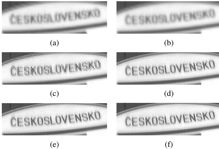
Figure 10.29 Super-resolution results using a variety of image priors (Capel 2001): (a) Low-res ROI (bicubic 3 \times zoom); (b) average image; (c) MLE @ 1.25 \times pixel-zoom; (d) simple \|x\|^2 prior ( \lambda = 0.004 ); (e) GMRF ( \lambda = 0.003 ); (f) HMRF ( \lambda = 0.01 , \alpha = 0.04 ). 10 images are used as input and a 3 \times super-resolved image is produced in each case, except for the MLE result in (c).
