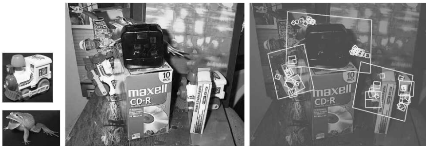
Figure 6.2 Recognizing objects in a cluttered scene (Lowe 2004) © 2004 Springer. Two of the training images in the database are shown on the left. They are matched to the cluttered scene in the middle using SIFT features, shown as small squares in the right image. The affine warp of each recognized database image onto the scene is shown as a larger parallelogram in the right image.
