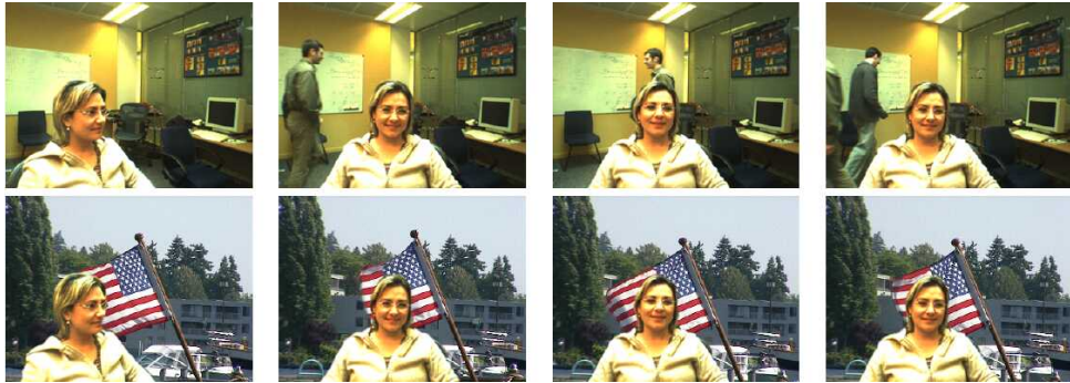
Figure 12.17 Background replacement using z-keying with a bi-layer segmentation algorithm (Kolmogorov, Criminisi et al. 2006) © 2006 IEEE.
