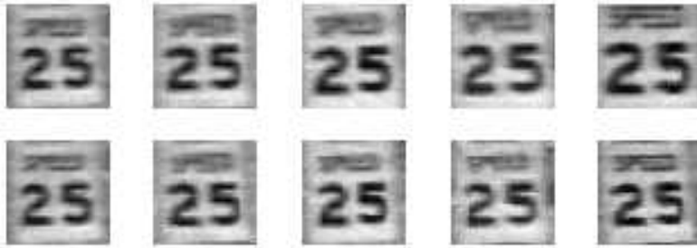
Figure 7.29 Feature tracking using an affine motion model (Shi and Tomasi 1994) © 1994 IEEE, Top row: image patch around the tracked feature location. Bottom row: image patch after warping back toward the first frame using an affine deformation. Even though the speed sign gets larger from frame to frame, the affine transformation maintains a good resemblance between the original and subsequent tracked frames.
