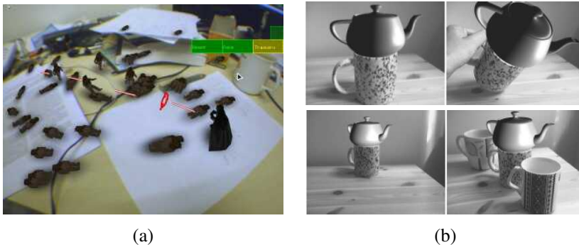
Figure 11.27 3D augmented reality: (a) Darth Vader and a horde of Ewoks battle it out on a table-top recovered using real-time, keyframe-based structure from motion (Klein and Murray 2007) © 2007 IEEE; (b) a virtual teapot is fixed to the top of a real-world coffee cup, whose pose is re-recognized at each time frame (Gordon and Lowe 2006) © 2007 Springer.
