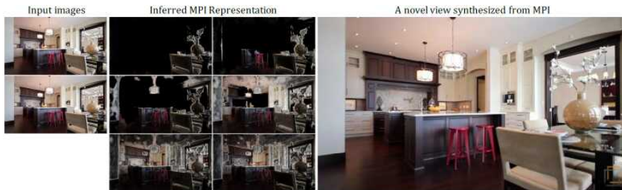
Figure 14.8 MPI representation constructed from a stereo pair of color images, along with a novel view reconstructed from the MPI (Zhou, Tucker et al. 2018) © 2018 ACM. Note how the planes slice the 3D scene into thin layers, each of which has colors and full or partial opacities in only a small region.
