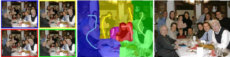
Figure 4.16 An unordered label MRF (Agarwala, Dontcheva et al. 2004) © 2004 ACM: Strokes in each of the source images on the left are used as constraints on an MRF optimization, which is solved using graph cuts. The resulting multi-valued label field is shown as a color overlay in the middle image, and the final composite is shown on the right.
