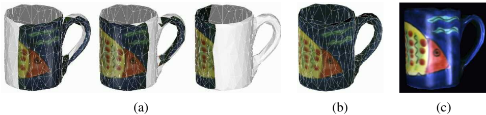
Figure 13.31 Estimating the diffuse albedo and reflectance parameters for a scanned 3D model (Sato, Wheeler, and Ikeuchi 1997) © 1997 ACM: (a) set of input images projected onto the model; (b) the complete diffuse reflection (albedo) model; (c) rendering from the reflectance model including the specular component.
