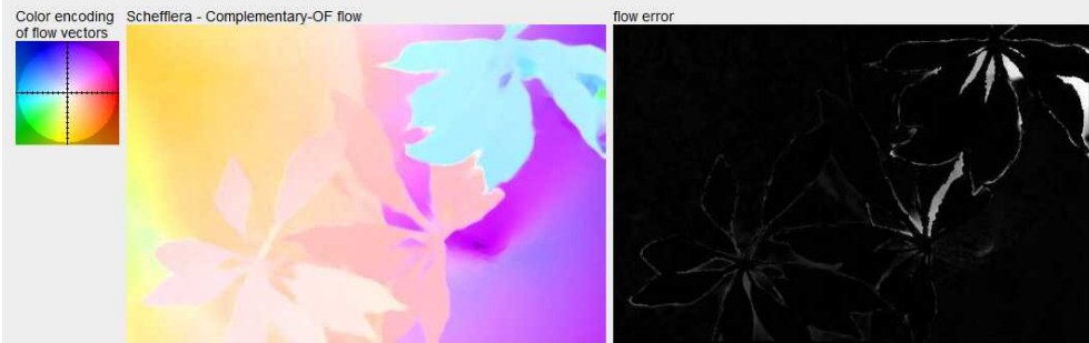
Figure 9.8 Evaluation of the results of 24 optical flow algorithms, October 2009, https://vision.middlebury.edu/flow/ , (Baker, Scharstein et al. 2009). By moving the mouse pointer over an underlined performance score, the user can interactively view the corresponding flow and error maps. Clicking on a score toggles between the computed and ground truth flows. Next to each score, the corresponding rank in the current column is indicated by a smaller blue number. The minimum (best) score in each column is shown in boldface. The table is sorted by the average rank (computed over all 24 columns, three region masks for each of the eight sequences). The average rank serves as an approximate measure of performance under the selected metric/statistic.
