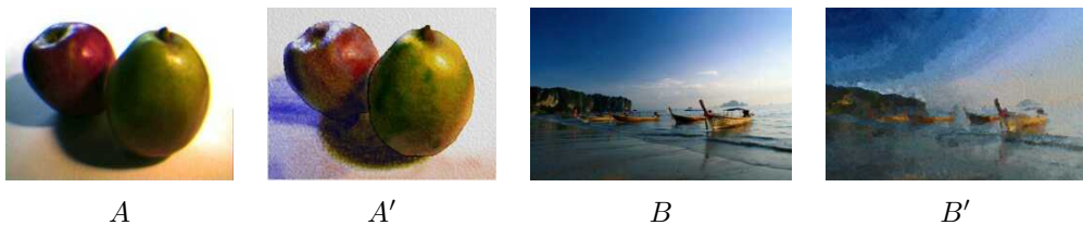
Figure 10.54 Image analogies (Hertzmann, Jacobs et al. 2001) © 2001 ACM. Given an example pair of a source image A and its rendered (filtered) version A' , generate the rendered version B' from another unfiltered source image B .
