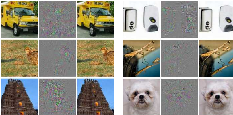
Figure 5.50 Examples of adversarial images © Szegedy, Zaremba et al. (2013). For each original image in the left column, a small random perturbation (shown magnified by 10\times in the middle column) is added to obtain the image in the right column, which is always classified as an ostrich.
