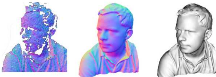
Figure 13.13 Fusing multiple depth images using the KinectFusion real-time system (Newcombe, Izadi et al. 2011) © 2011 IEEE. The three images show an original (noisy) range scan, rendered as a colored normal map, and the fused 3D model, rendered as both a normal map and Phong-shaded.
