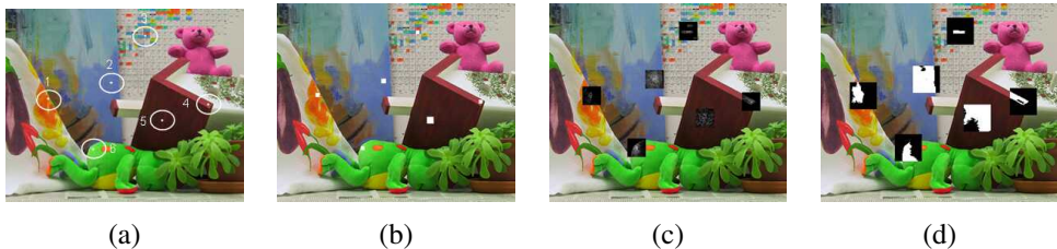
Figure 12.10 Aggregation window sizes and weights adapted to image content (Tombari, Mattoccia et al. 2008) © 2008 IEEE: (a) original image with selected evaluation points; (b) variable windows (Veksler 2003); (c) adaptive weights (Yoon and Kweon 2006); (d) segmentation-based (Tombari, Mattoccia, and Di Stefano 2007). Notice how the adaptive weights and segmentation-based techniques adapt their support to similarly colored pixels.
