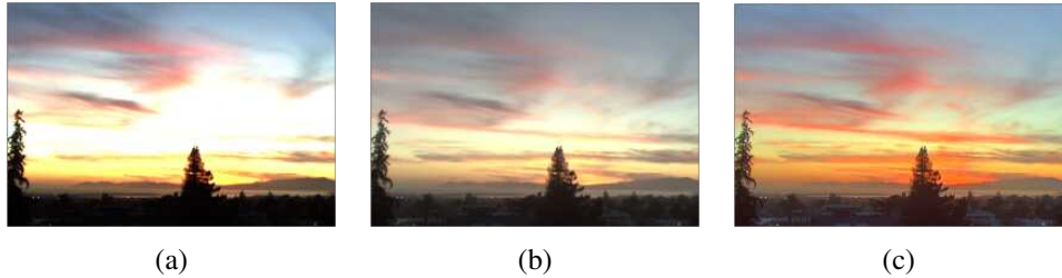
Figure 10.18 Global tone mapping: (a) input HDR image, linearly mapped; (b) gamma applied to each color channel independently; (c) gamma applied to intensity (colors are less washed out). Original HDR image courtesy of Paul Debevec, https://www.pauldebevec.com/Research/HDR . Processed images courtesy of Frédo Durand, MIT 6.815/6.865 course on Computational Photography.
