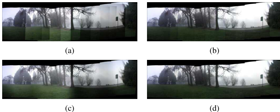
Figure 10.6 Simultaneous estimation of vignetting, exposure, and radiometric response (Goldman 2010) © 2011 IEEE: (a) original average of the input images; (b) after compensating for vignetting; (c) using gradient domain blending only (note the remaining mottled look); (d) after both vignetting compensation and blending.
