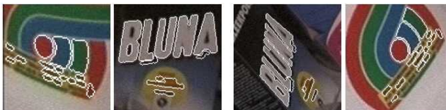
Figure 7.14 Maximally stable extremal regions (MSERs) extracted and matched from a number of images (Matas, Chum et al. 2004) © 2004 Elsevier.
