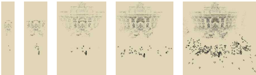
Figure 11.17 Incremental structure from motion (Snavely, Seitz, and Szeliski 2006) © 2006 ACM. Starting with an initial two-frame reconstruction of Trevi Fountain, batches of images are added using pose estimation, and their positions (along with the 3D model) are refined using bundle adjustment.
