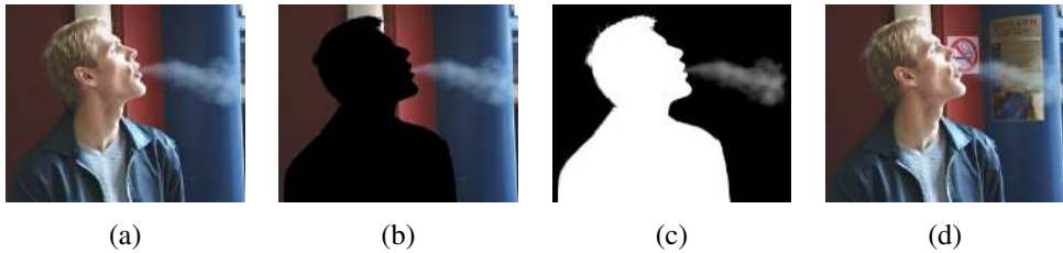
Figure 10.47 Smoke matting (Chuang, Agarwala et al. 2002) © 2002 ACM: (a) input video frame; (b) after removing the foreground object; (c) estimated alpha matte; (d) insertion of new objects into the background.
