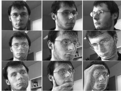
Figure 7.30 Real-time head tracking using fast trained classifiers (Lepetit, Pilet, and Fua 2004) © 2004 IEEE.
