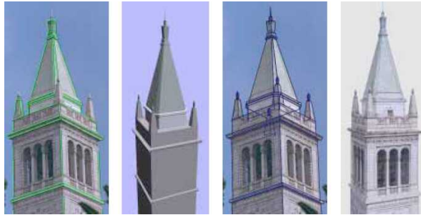
Figure 13.19 Interactive architectural modeling using the Façade system (Debevec, Taylor, and Malik 1996) © 1996 ACM: (a) input image with user-drawn edges shown in green; (b) shaded 3D solid model; (c) geometric primitives overlaid onto the input image; (d) final view-dependent, texture-mapped 3D model.
