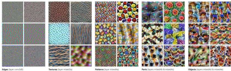
Figure 5.49 Feature visualization of how GoogLeNet (Szegedy, Liu et al. 2015) trained on ImageNet builds up its representations over different layers, from Olah, Mordvintsev, and Schubert (2017).
