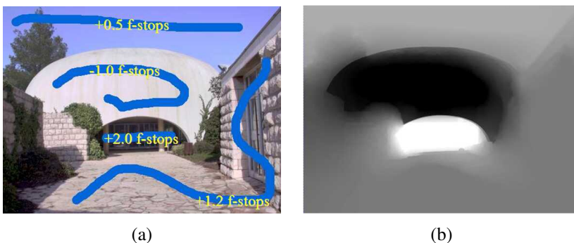
Figure 10.26 Interactive local tone mapping (Lischinski, Farbman et al. 2006) © 2006 ACM: (a) user-drawn strokes with associated exposure values g(x, y) ; (b) corresponding piecewise-smooth exposure adjustment map f(x, y) .
