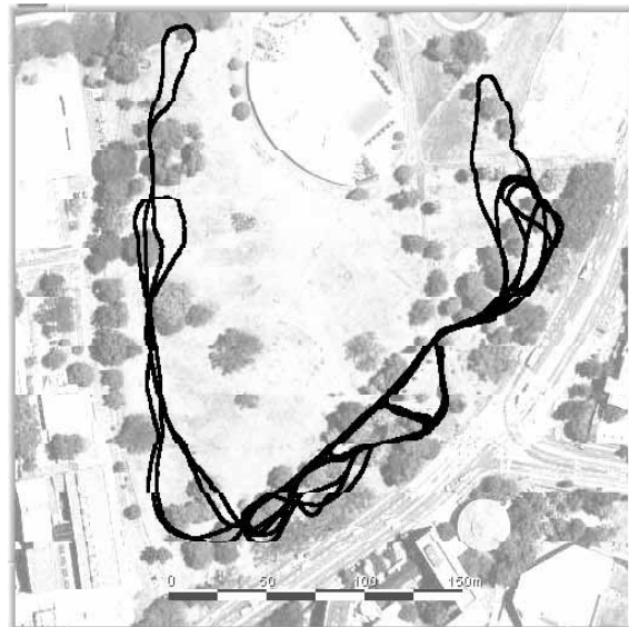
Figure 12.15 The path recovered by the SEIF, is correct within \pm 1m . Courtesy of Michael Montemerlo, Stanford University.
