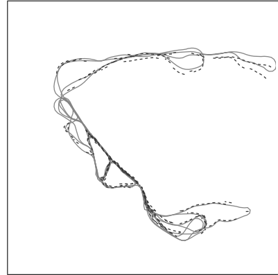
(b) FastSLAM 1.0 (solid), GPS path (dashed)
