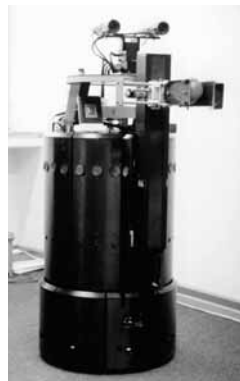
Figure 9.12 Mobile indoor robot of the type RWI B21, with 24 sonar sensors mounted on a circular array around the robot.
