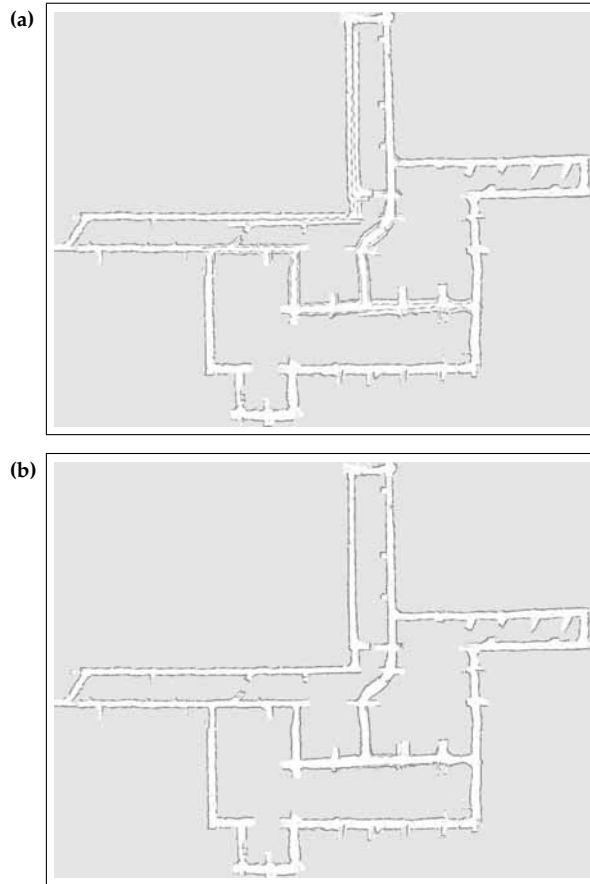
Figure 12.18 (a) Map with incremental ML scan matching and (b) full recursive branch-and-bound data association. Images courtesy of Dirk Hähnel, University of Freiburg.
